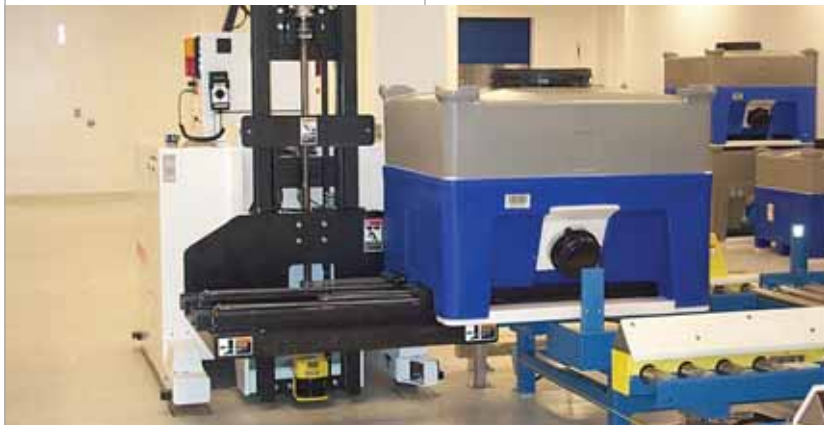
A self-guided vehicle picks up a tote from a conveyor, which rests on load cells. Photo courtesy of Apotex, Inc.
