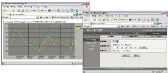
Incorporating TandD's proprietary ProDigio web server chipset, the TR-7xW products contain an HTTP server for device connectivity to the web. This permits device configuration, reading of current values or downloading of logged data with a standard web browser from any PC connected to the internet, anywhere in the world. Recorded
