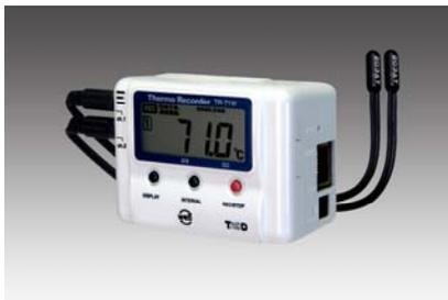
The TR-71W is a two-channel temperature data logger capable of storing 8,000 readings for each channel. The sampling rate can be set to any of 15 intervals, from once per second to once per hour, in either two recording modes. In one time mode the unit will take readings until the memory is full and then stop. In endless loop mode the unit will “wrap around” in memory once it is full and overwrite the oldest data. The TR-71W ships with
