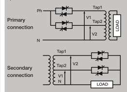
The operating region of control will determine the number of taps required but a maximum of 4 is usually sufficient.
